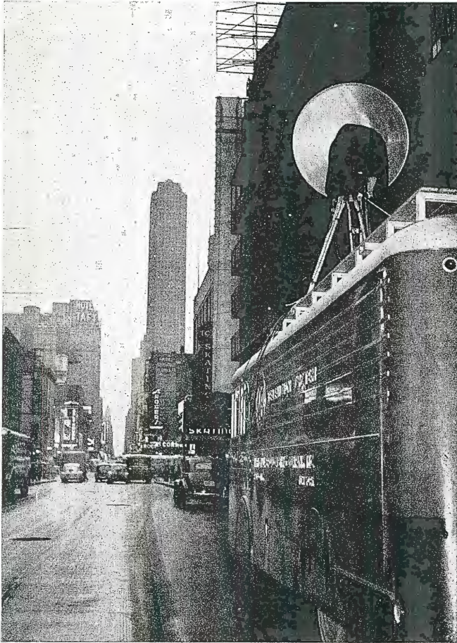
FIG. 4. The microwave antenna atop the telemobile unit parked beside Madison Square Garden. The antenna is directed toward the top of the RCA Building shown in the center of the photo.
