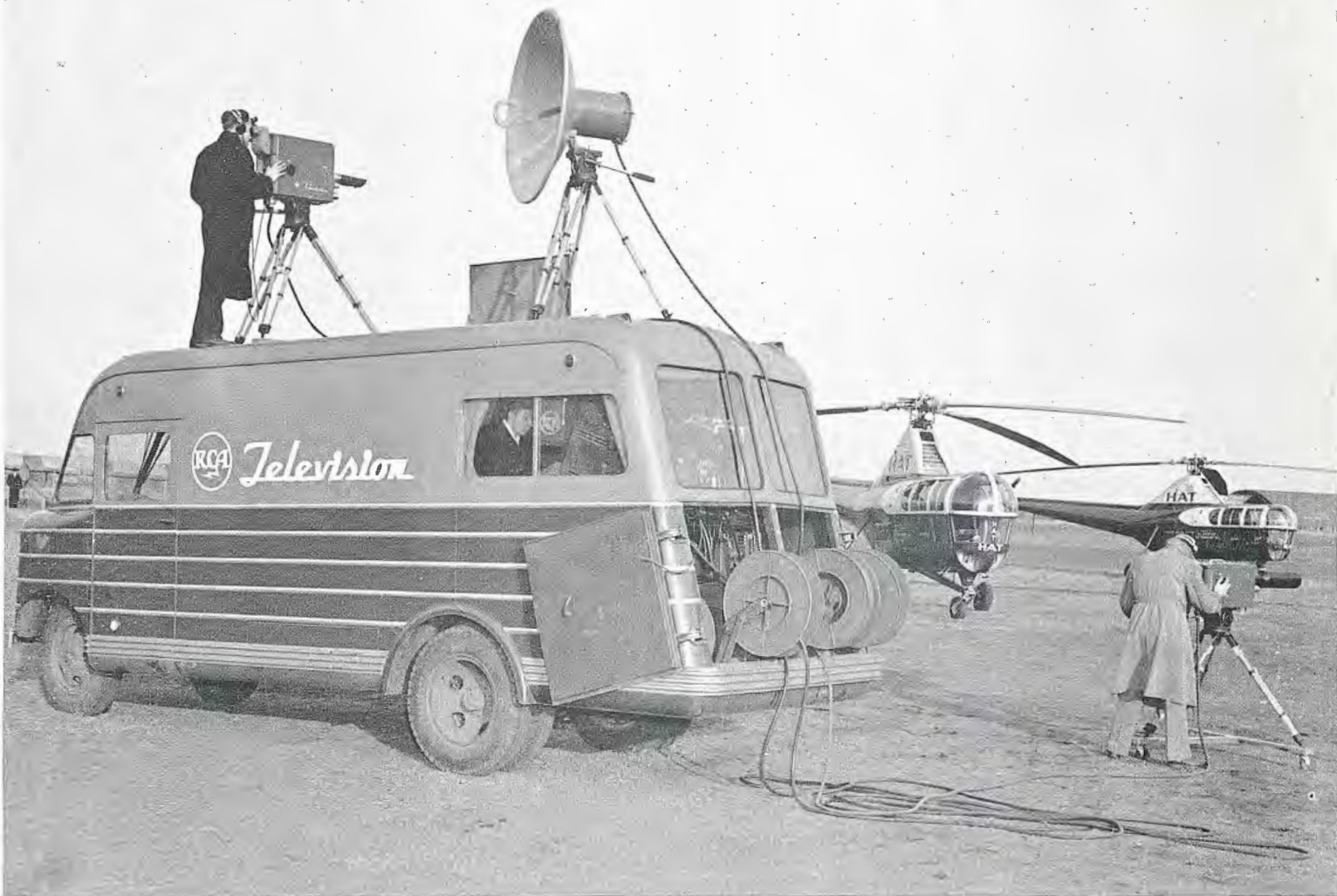
FIG. 1. The TJ-50A Mobile Unit (shown here at Camden Airport) provides both transportation and control space for standard field equipment. Cameras may be operated from the roof of the unit or placed as much as 1000 feet away.
