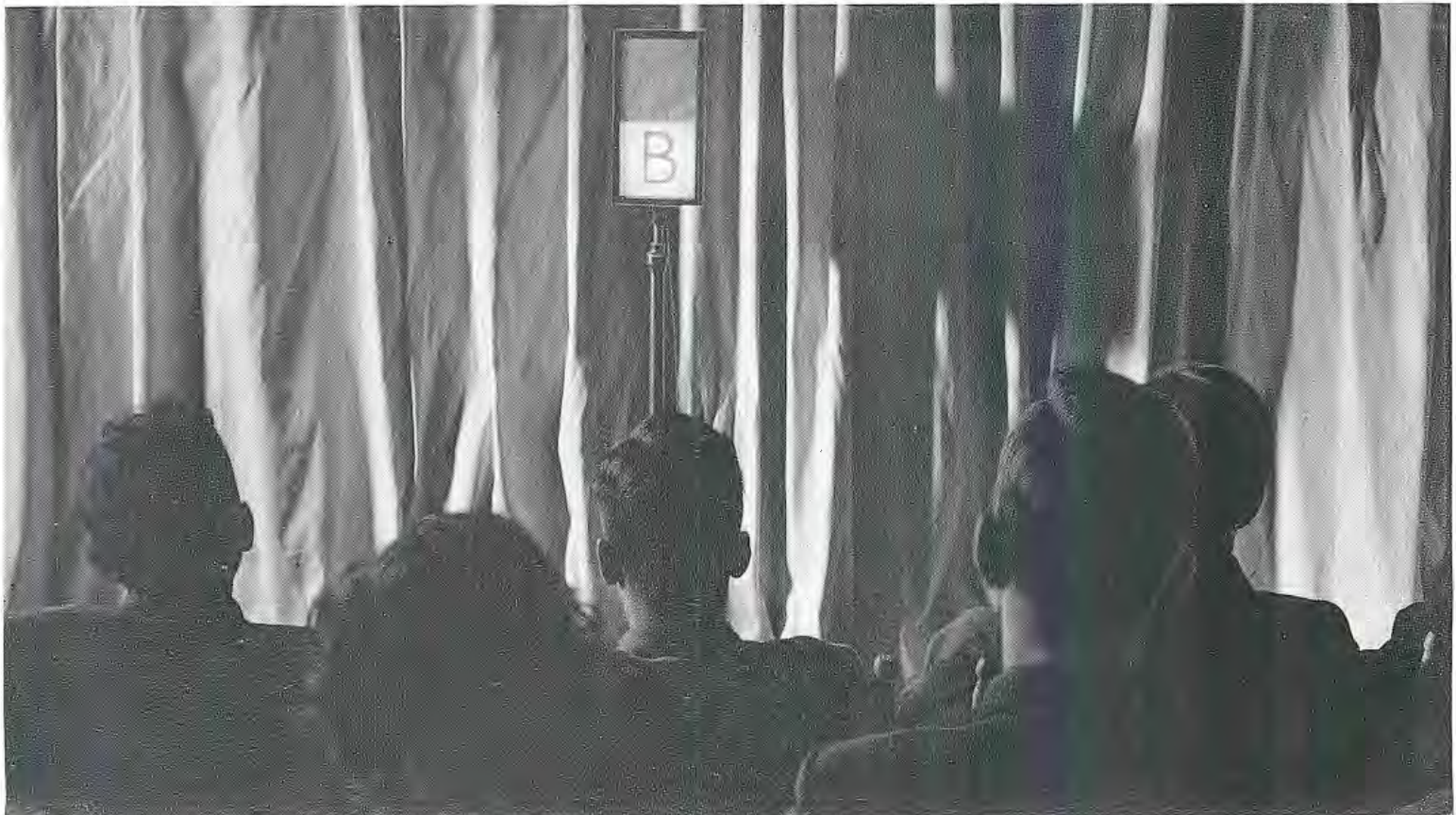
FIG. 7. Cloth curtain in front of filter prevents listeners from seeing position of the vanes.
