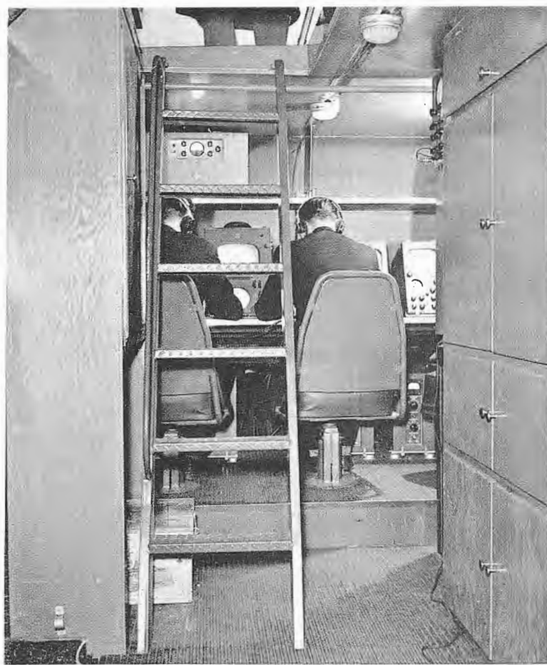
FIG. 3. (left) View inside the mobile unit, looking from the driver's seat toward the rear. Ladder, which provides easy access to the roof hatch, folds to ceiling when not in use. Cabinets at right provide carrying space for cameras, relay equipment, etc.
