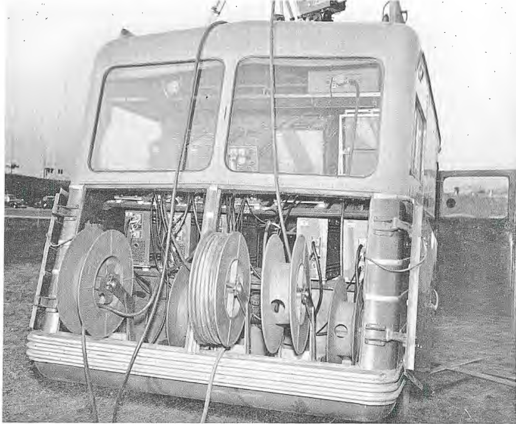
FIG. 7. (left) Rear view of unit showing how cable reels can be pulled out to facilitate unreeling. Inner end of cable extends through hole in reel to receptacle on camera control units on the operating table just above.
