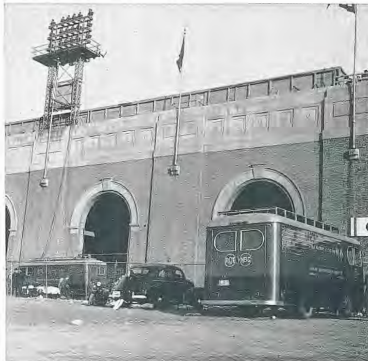
FIG. 3. The two telemobile units parked outside the stadium. Note cables running from unit at left up over stadium wall. The unit at right was used for transportation only.
