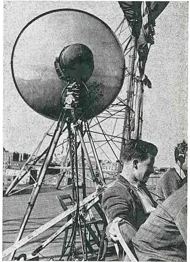
FIG. 5. Atop the grandstand at Ebbets Field, Brooklyn, the RCA Microwave transmitting parabola antenna lined up for a direct relay to the RCA Building.
